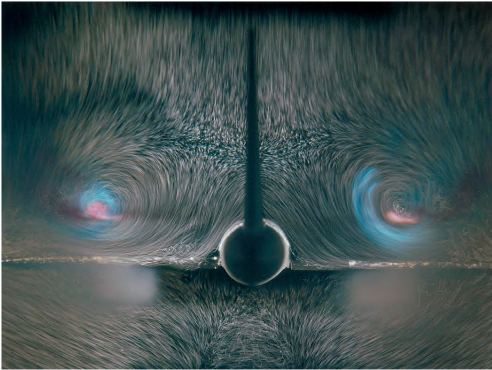
Figure 3.10: Laser-sheet visualization of the streamlines of the transverse flow around the Concorde. (ONERA image.)
